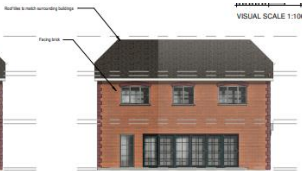
③ PR 02. Building-A. Rear Elevation 1 : 100
