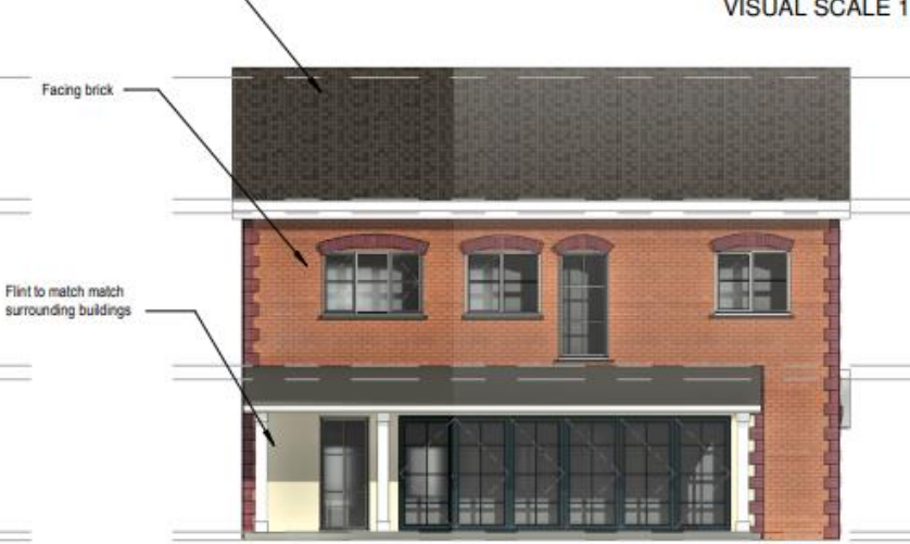
③ PR 02. Building-A. Rear Elevation 1 : 100
