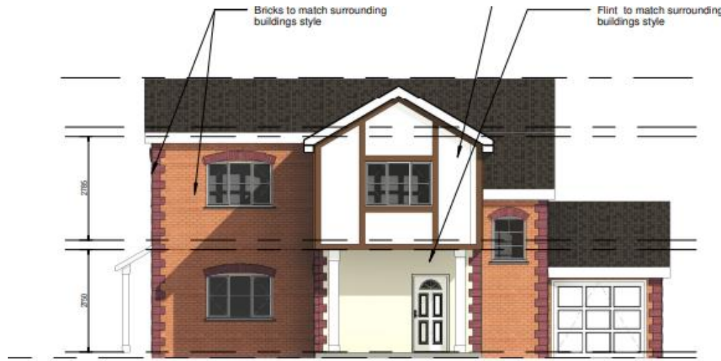
① PR 01. Building - B. Front elevation 1 : 100
